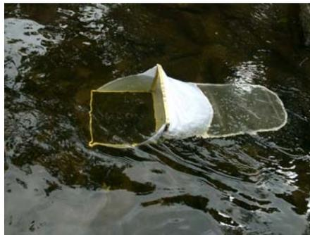
Figure 2: Surber Bottom Sampler
