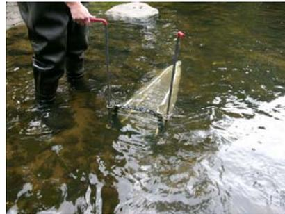
Figure 3b: Drift net in the water
