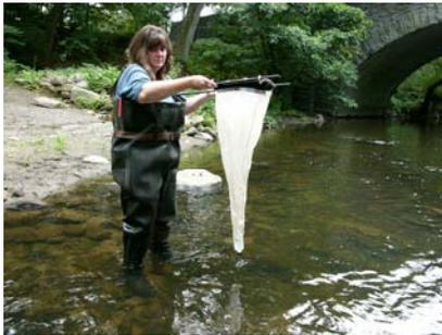
Figure 3a: Drift net showing cod end.
